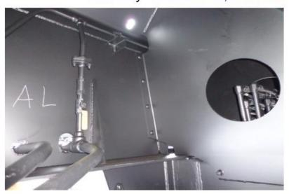
The ball valve located at the AL corner of the car directly above the AL side bearing must be in the open position to allow the supply air to the door valve assembly. This valve is normally in the open position and is used to stop the supply air to the door valve if there is an issue that requires air to be discontinued to a subject car without interrupting air supply to the other cars in the consist.
