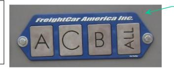
Touch Pad Ground Plate Aluminum ground plate around Touch Pad assembly
