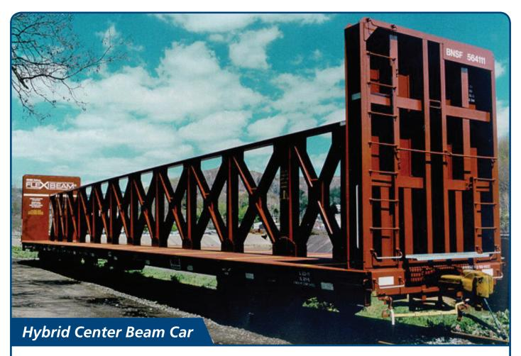
FreightCar America's FlexiBeam™ center beam car is the optimal car for hauling a variety of forest and steel products. FlexiBeam is an all welded, 100-ton capacity flatcar with end bulkheads and a girder of tubular beam construction on the longitudinal centerline. The car has a 286,000 pound gross rail load.
