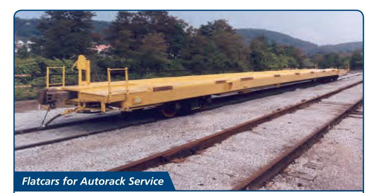
These 89' cars include 70-ton flush deck flatcars for application of bi-level autoracks and 70-ton low-level flatcars designed for tri-level autorack service. The flat cars feature all steel, welded designs and are custom built to meet specific customer require-
